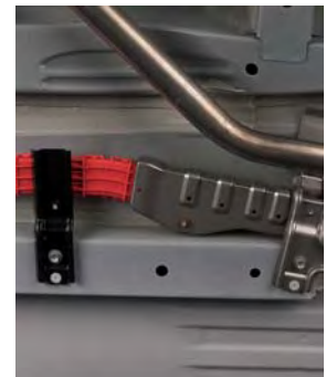
Thermal shield near hot exhaust
