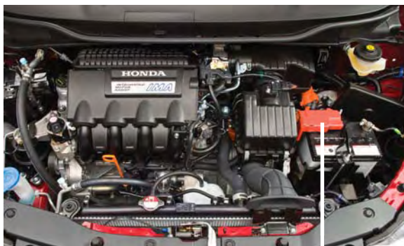
Positive Battery Terminal
