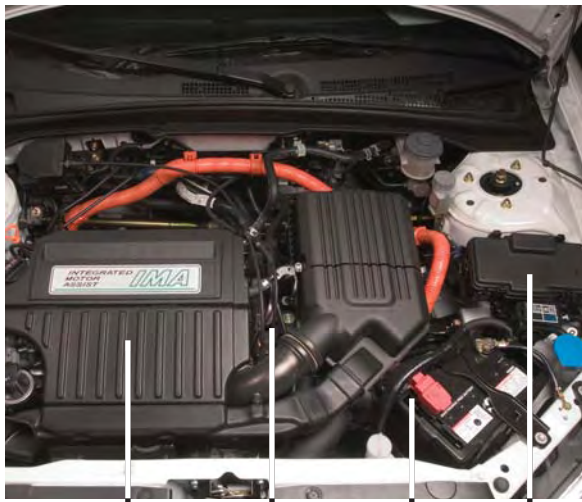
Engine Motor 12-Volt Battery Underhood Fuse Box
