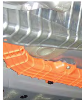
Electrical shield bolted to undercarriage
